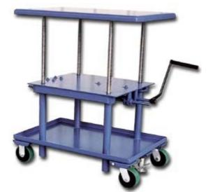
This adjustable height portable table is well suited for a wide variety of material handling applications. Mechanical crank mechanism provides positive height adjustment without downward drift. Two speed gear mechanism moves loads at 1/8" per crank rotation and light loads at 3/8" per crank rotation.  $5" \times 2"$  two rigid/two swivel polyurethane casters and floor lock standard.
